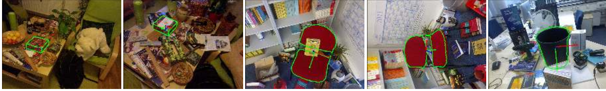
Figure 7. Example scenes and detection results for several example scenes with high amounts of clutter and occlusion. The detections are outlined in green. Note that for objects that were reconstructed from reference images, such as the chair, have a rather rough outline compared to objects modeled with CAD, such as the box.
