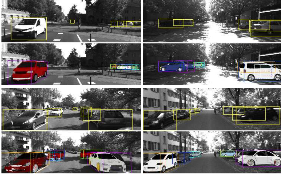
Figure 8: KITTI: examples of car detections. ( top ) Ground truth, ( bottom ) Our 3D detections, augmented with best fitting CAD models to visualize inferred 3D box orientations.
