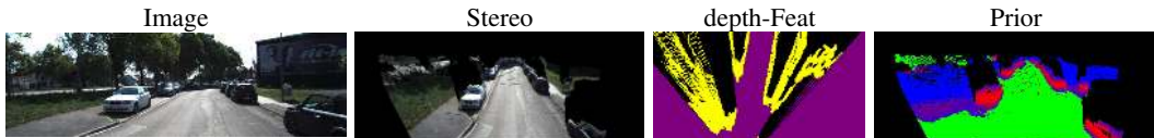
Figure 1: Features: From left to right: original image, stereo reconstruction, depth-based features and our prior. In the third image, purple is free space ( F in Eq. (2)) and occupancy is yellow ( S in Eq. (1)). In the prior, the ground plane is green and red to blue indicates distance to the ground.
