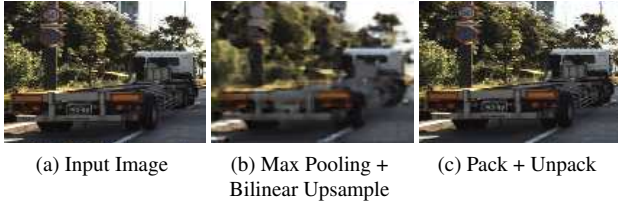
Figure 4: Image reconstruction using different encoder-decoders: (b) standard max pooling and bilinear upsampling, each followed by 2D convolutions; (c) one packing-unpacking combination (cf. Fig. 3) with D = 2 . All kernel sizes are K = 3 and C = 4 for intermediate channels.
