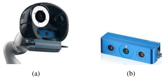
Figure 1: Acquisition system: (a) Robot with its vision-based sensory system, (b) Ensenso N35 3D scanner
