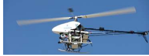
Fig. 2. COLIBRI III Electric helicopter UAV used for pose estimation tests.
