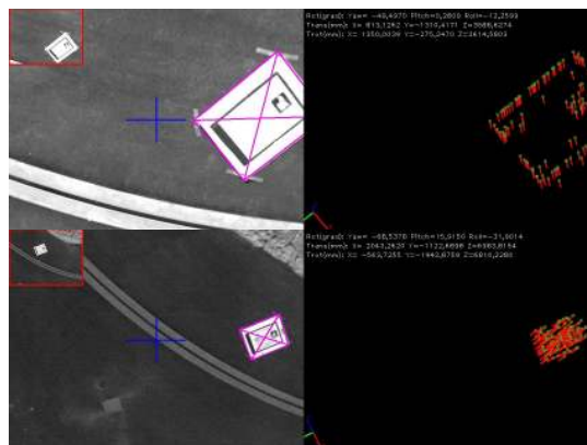
Fig. 6. Two different test for 3D pose estimation based on a helipad tracking using Robust Homography estimation. Up: Flight test beginning at an altitude of 4.2m . Down: Flight test beginning at an altitude of 10m . In both images, the reference image I_0 is on the small rectangle on the upper left corner. Left it the current frame and Right the Optical Flow between the actual and last frame. Superimposed are the projection of the original rectangle, the translation vector and the Tait-Bryan angles.
