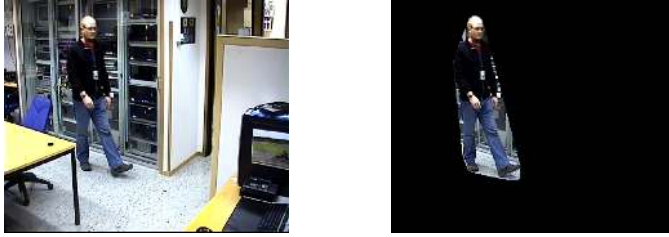
(a) A frame before the foreground segmentation. (b) The same frame after the foreground segmentation.
