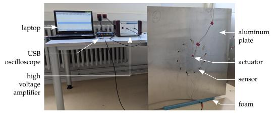
Figure 3. Test setup to determine the peak-to-peak voltage of the sensors under GUW excitation.
