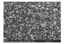
**Figure 1.** Scanning Electron Microscopy image of 20 vol% PZT/photopolymer composite shows homogeneous particle dispersion and no agglomerations.
