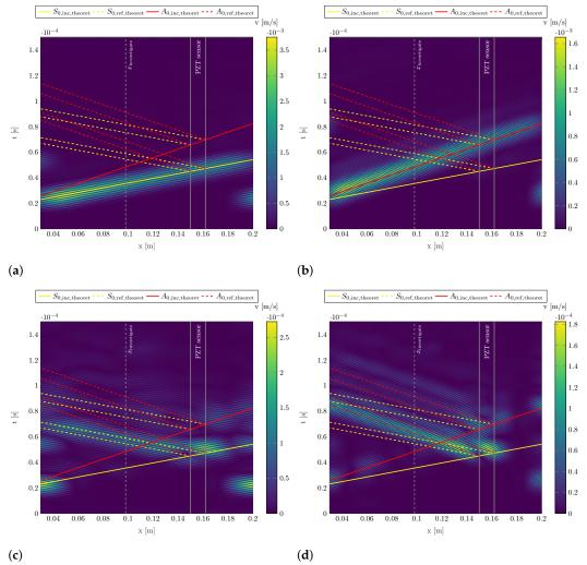
**Figure 8.** Filtered B-scans for identifying incident and reflected  $S_0$  and  $A_0$  modes for an excitation with a burst center frequency of  $f_c = 300$  kHz. 2 mm aluminum plate with surface-applied PZT ceramic. (a) Filtered incident  $S_0$  mode from in-plane data. (b) Filtered incident  $A_0$  mode from out-of-plane data. (c) Filtered reflected  $S_0$  mode from in-plane data. (d) Filtered reflected  $A_0$  mode from out-of-plane data.
