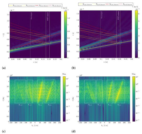
**Figure 7.** B-scans and two-dimensional spatial-temporal Fourier transformation of three-dimensional SLDV data at  $f_c = 300$  kHz in the 2 mm aluminum plate along the measuring path containing the PZT sensor (Figure 2b). (a) B-Scan (In-plane component). (b) B-Scan (Out-of-plane component). (c) Two-dimensional FFT of in-plane data (Quadrants 1 and 4). (d) Two-dimensional FFT of out-of-plane data (Quadrants 1 and 4).
