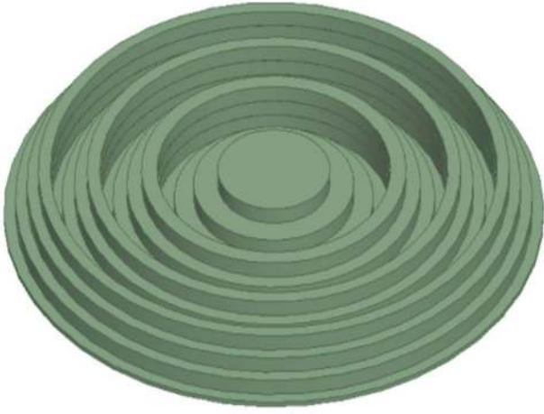
Fig. 1 3D schematic view of lens composed of 4 quarter wave zones and 4 step heights
