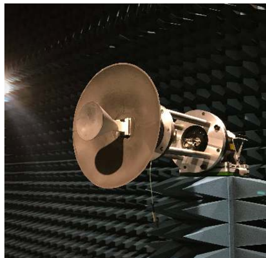
FIGURE 14. 3D-printed dual-reflector antenna with the proposed subreflector in the measurement chamber.
