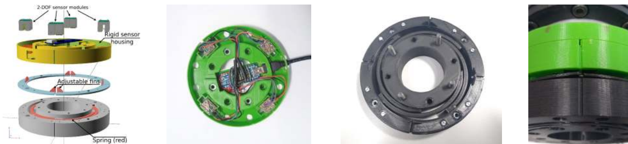
FIGURE 22. Six-axis F/T sensor using eight fork-type interrupters and adjustable fins; d = 104 mm, F_x, F_y, F_z = 20 N. (a) OpenSCAD rendering with the key parts (top to bottom): four 2-DOF sensor modules and microcontroller, fixed upper ring with sensor housings, four quarter-circle sheets with adjustable 45-degree fins, moving tool-mounting ring with spiral spring. (b) Upper ring with sensor-modules and microcontroller. (c) Base ring with spiral spring and adjustable fins installed. (d) Close-up view of two adjusted fins on the assembled sensor.
