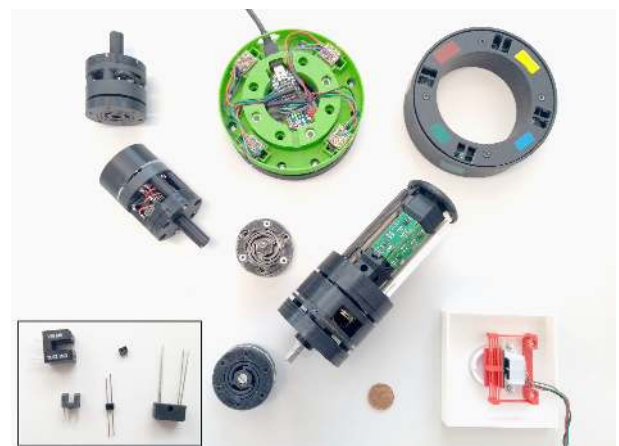
FIGURE 1. A family of 3D printed low-cost force-sensing objects, based on proximity- or interrupter-type optical sensors (inset on bottom left). The examples in the figure range from a 2-DOF friction-force sensor for object pushing experiments to 6-DOF force/torque sensors with different sizes, shapes, and sensitivity. Also shown is a 17-DOF force/torque-sensing screwdriver for learning from human demonstration.
