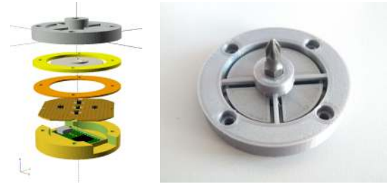
FIGURE 20. (a) CAD model of the tool part with 1/4 inch bit holder and five reflex-type sensors. (b) Bit holder elastic element with Pozidriv bit; note thin double levers and quarter-circle overload end stops.
