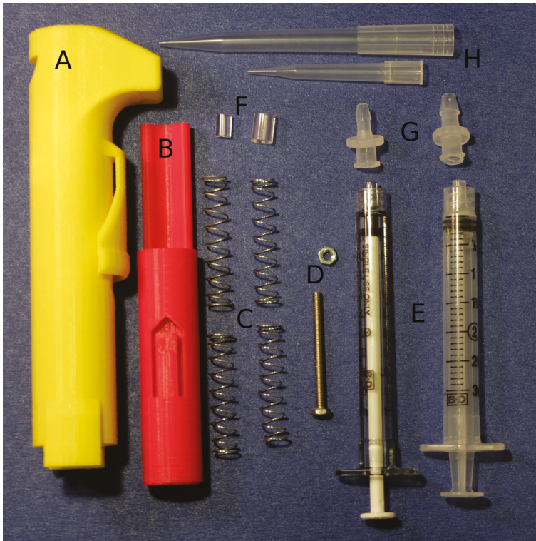
Figure 3. Photo of the parts to make the pipette. (A) Printed body part. (B) Printed plunger part. (C) Springs. (D) M3 hex nut and M3 bolt. (E) Disposable syringes. (F) Two sizes of tubing to adapt pipette tips to luer barb. (G) Luer lock syringe-to-barb adapters. (H) Pipette tips. A list of parts is in Appendix A: Tables A1 and A2.
