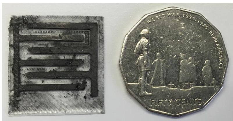
Figure 5: Comparison of the size of the sensor patch with a 50 cent AUD.
