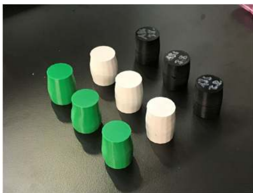
Fig. 4 FDM AM material variation: PETG (green), PLA (white), and ABS (black). Cylindrical specimens are subjected to compression tests to evaluate the mechanical properties of the material
