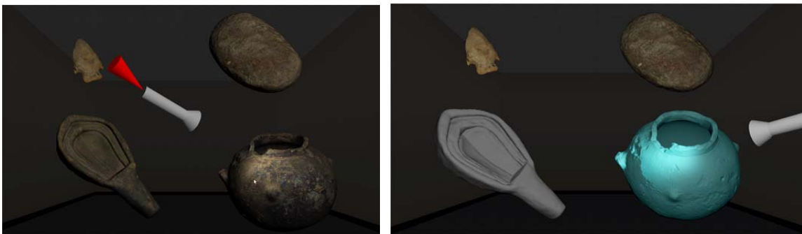
Figure 3. Highlight of object manipulation and visualization in the Powerwall in dark environmental light condition. The red cone represents the user's pointer designed to interact with the scene (objects and menu 3D interaction and lights repositioning). Left: The user is moving the light source to enhance objects details. Right: similar situation where the objects textures were removed to analyze the polygonal representation.
