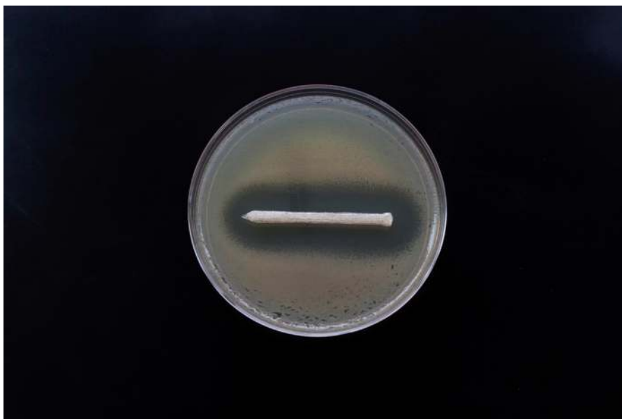
Figure 13. Zone of inhibition of 3D printed PLA–GS pin.
