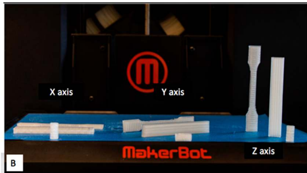
Figure 1. 3D Printed polylactic acid (PLA) constructs (compression cylinders, flexural bars and dog-bone shape) in different orientations.
