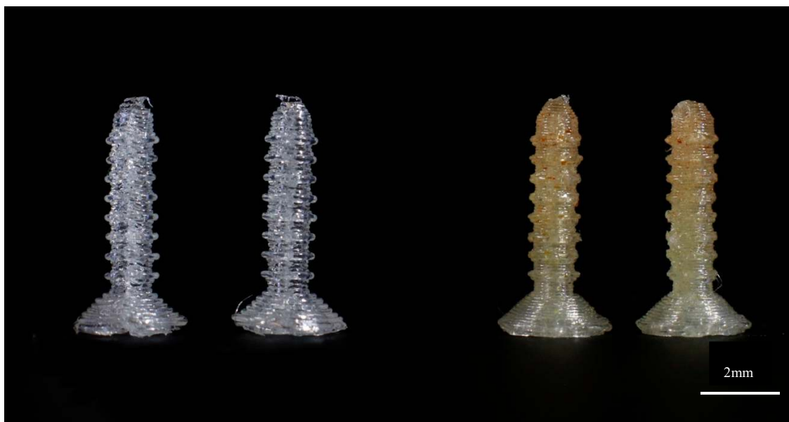
Figure 4. 3D printed standard 4 mm screws using control PLA and PLA-GS.
