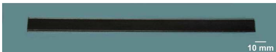
Figure 5. Sample with 6 layers of CFRTP printed by the Mark One ® . The sample still has to be ground and the tabs still have to be attached.
