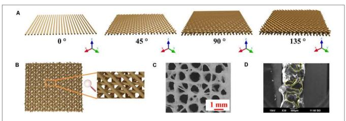
FIGURE 5 | 3D printing schema. (A) Schematic of fabrication of multi-angle 3D printed Alg/Gel scaffold. (B) Top view of four-layer model of 3D printed Alg/Gel scaffold. (C) Photomicrograph of top view of freeze-dried multi-angle 3D Alg scaffold. (D) SEM image of cross-sectional view of 3D Alg scaffold with horizontal pores highlighted by yellow contours.
