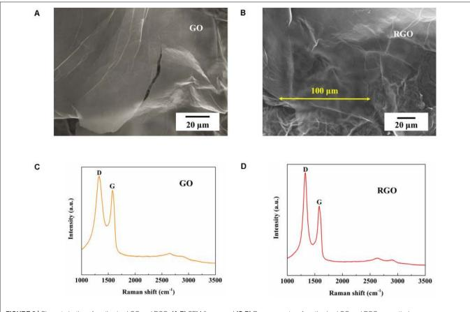
FIGURE 3 | Characterization of synthesized GO and RGO. (A,B) SEM figures and (C,D) Raman spectra of synthesized GO and RGO respectively.
