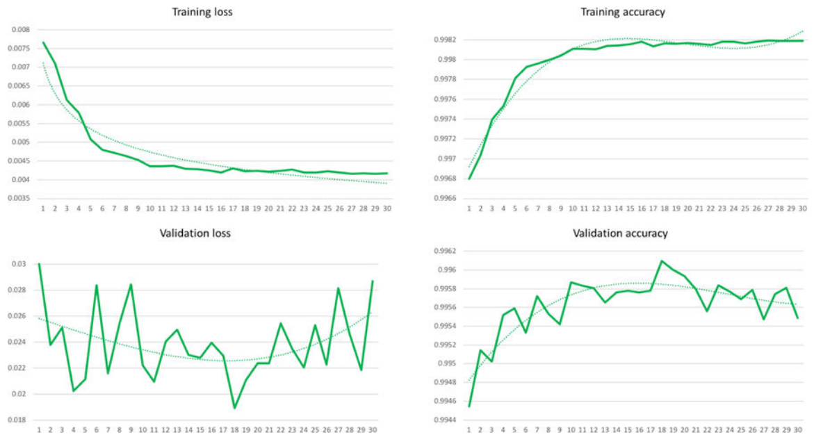
Fig. 7. Training and validation loss and accuracy curves and fitted polynomial trendline as a function of epochs. Over-fitting is observed after epoch 20.
