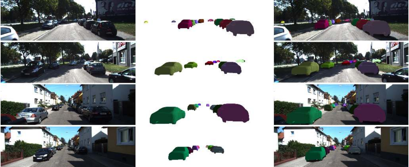
Figure 6: Qualitative demonstration of our approach working on KITTI [13] dataset. Input images are shown in first column, and the corresponding 3D object pose and shape output are shown in second column. Each object instance has been colored randomly. Third column shows the projection of the 3D object instance reconstructions on the input image which demonstrates the capability of producing accurate 2D instance segmentation, which comes for free due our holistic 3D representation.
