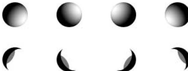
Figure 30. Examples of non-conservative shadow estimates. Upper row: Examples of self-shadows cast over the surface of a sphere. Lower row: The corresponding shadow estimates are shown in black; the lit areas misclassified as shadows are in gray.
