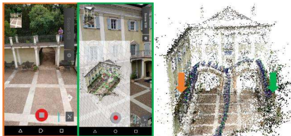
Figure 2: Example of on-the-fly visual feedback inside the smartphone's app (left) during a collaborative digitization process (here two users involved) or on the web browser (right).
