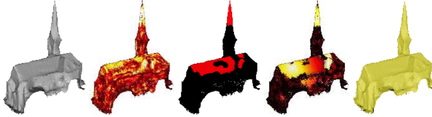
Figure 3. Our pipeline (shown on one object extracted from the city-scale point cloud). Left to right: Input, landmark score \mathcal{L} , components \mathcal{C} , refined landmark score \mathcal{L}^* , building aggregation. The color changes from black (low) to white (high score).
