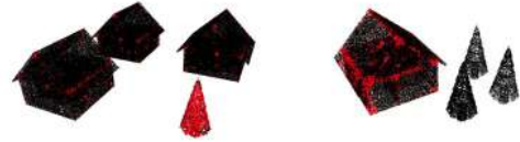
Figure 2. Context-dependency of the notion of landmark, illustrated with our distinctiveness measure for landmarks (red points). Left: almost all unique points belong to the tree since houses are common. Right: the majority of unique features belong to the house as trees are common.
