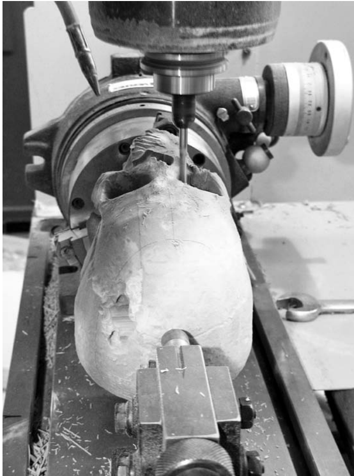
Fig. 2. CNC milling of replica of 17th century human skull from an archaeological site, part of a forensic reconstruction of the individual for a museum display (By Carolyn Thome, Office of Exhibits Central, courtesy of Smithsonian Institution)
