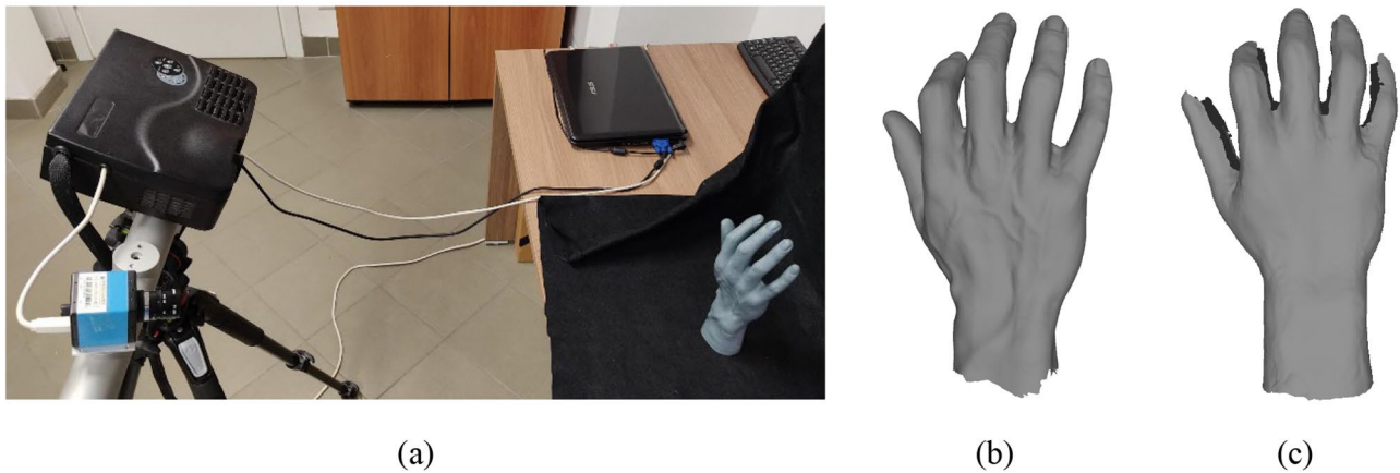
Fig. 7 Acquisition of the plaster hand: (a) setup of the stationary scanner, (b) 3D mesh obtained with the stationary scanner, and (c) with the developed hand-held scanner
