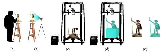
**Figure 10.** Basic steps of 3D scanning/printing: (**a**) creation of physical model; (**b**) 3D scanning; (**c**) 3D printing in layers; (**d**) 3D printing by removing the material from a mass; (**e**) production of the artifact to any scale with marble, metal or synthetic materials.
