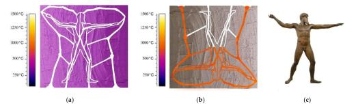
**Figure 5.** Basic steps of lost-wax casting method: (a) the fire-resistant mortar with the wax model and wax-tubes network is heated to 250-350 °C for 3-15 days (depending on the size of statue) and the wax is melted out; (b) metal foundry; (c) final artifact after the removal of metal tubes.
