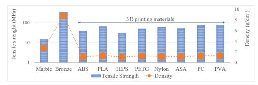
**Figure 11.** Evaluation of marble, bronze and common 3D printing materials. ABS: acrylonitrile butadiene styrene; PLA: polylactic acid; HIPS: high impact polystyrene; PETG: glycolized polyester; ASA: acrylonitrile styrene acrylate; PC: polycarbonate; PVA: polyvinyl alcohol.
