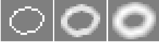
Figure 2: Example of “submanifold” dilation. Left: Original curve. Middle: Result of applying a regular 3 \times 3 convolution with weights 1/9 . Right: Result of applying the same convolution again. Regular convolutions substantially reduce the feature sparsity with each convolutional layer.
