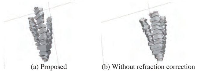
Fig. 7 3D reconstruction results. (a) 3D shape by proposed method. (b) 3D shape by SFS without refraction correction. Compared with (a), (b) is much thicker than the real 3D shape, due to the barrel-like distortion caused by the water tank.
