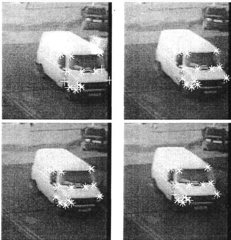
Figure 4. Originally detected (marked by x) and reconstructed (marked by +) corners overlaid on four frames of a van sequence.
