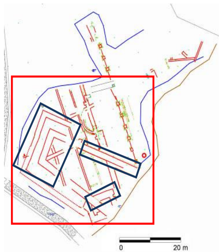
Figure 2. The site sketch produced from a total station survey showing the areas surveyed with UAV and TLS laser scanner (red) as well as with photogrammetry (blue).
