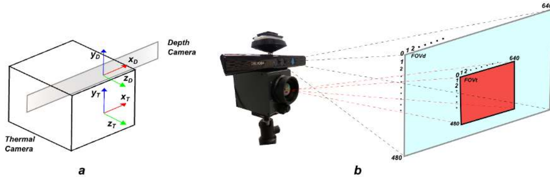
Figure 2: a: Stereo-multimodal system setup. b: Field of view (FOV) relationship between the cameras.
