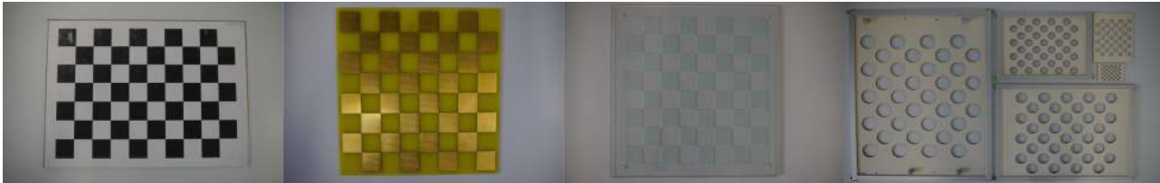
Figure 5. Various tested calibration targets. From left to right: Paper (chessboard), glass (chessboard), PCB (chessboard), laser-cut firm cardboard target (asymmetric circles).
