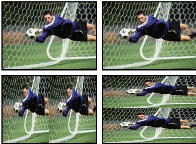
Fig. 1: Full Resolution (top) and Frame Compatible (bottom) representations of stereoscopic videos.
