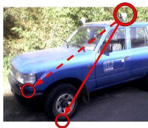
Fig. 8 Calibration of the wheel contact points of the survey vehicle, relative to the stereo rig
