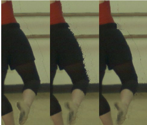
Fig. 4: Impact of depth coding artifacts on view synthesis rendering for Ballet sequence with uncoded color data: left : original uncoded depth, middle : H.264/MVC coded depth, and right Platelet coded depth.
