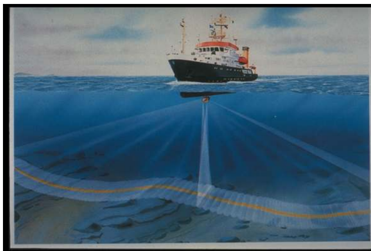
Figure 1. Typical geometry of bottom tracking multibeam sonar. A fan-shaped beam that is wide across track and narrow along track is transmitted while many receive beams that are narrow across track and wide along track are formed. The intersection of these beams (yellow boxes) results in many simultaneous depth measurements across the swath, each with excellent lateral resolution.
