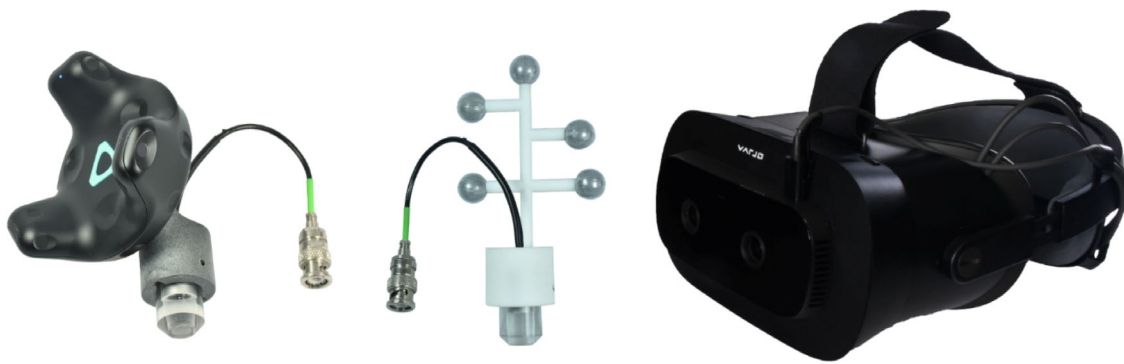
Fig. 1 Used hardware—UT sensors with different tracking hardware and Mixed Reality headset
