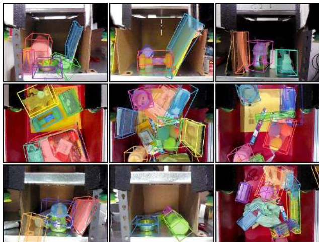
Figure 8. Predicted object poses on the Shelf & Tote Benchmark using 3DMatch + RANSAC. Predicted object poses are shown on the images of the scans with 3D bounding boxes of the transformed object models. 3DMatch + RANSAC works well for many cases; however, it may fail when there is insufficient depth information due to occlusion or clutter (bottom).
