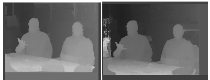
Figure 10: Disparity maps of the trifocal system: vertical baseline (left) and horizontal baseline (right)
