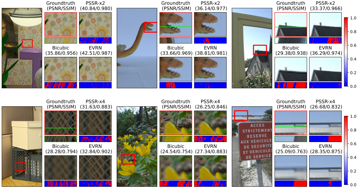
Figure 9: Comparison of two stages in reconstruction of spatially high resolution LF. The SAI at \theta = (4, 4) is visualized together with its zoom-in region marked by a red rectangle. For each approach, an EPI at horizontal line marked in green is extracted and compared to the EPI of Groundtruth. The first row, from left to right: \times 2 results of synthetic scene mona [8] and real-world scenes Ankylosaurus , Diplodocus_1 , Framed [14]. The second row, from left to right: \times 4 results of synthetic scene boxes [9] and real-world scenes Flowers , Sign [14].
