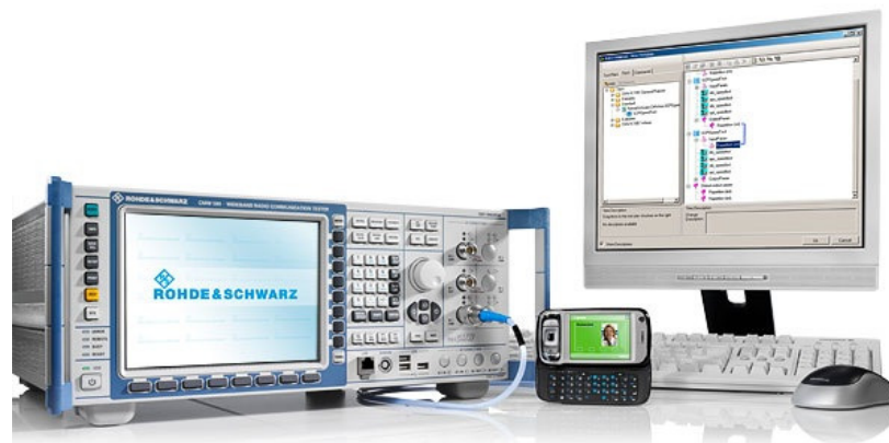
Figure 3.2: R&S CMW500 wideband radio communication tester [39].
