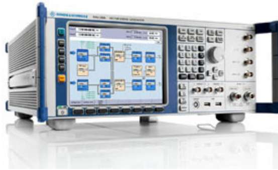
Figure 3.3: R&S AMU200A signal generator and fading simulator [39].
