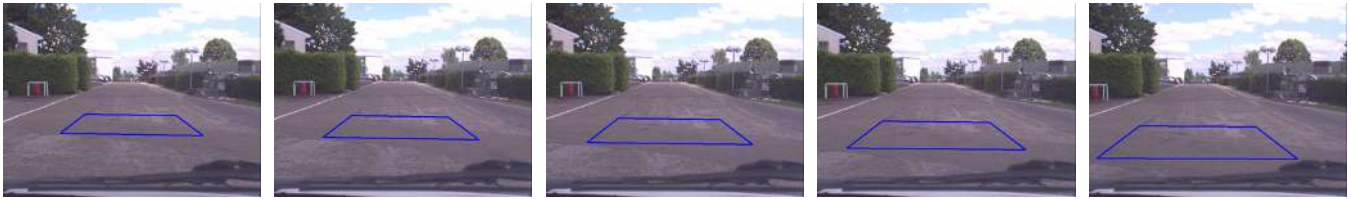
Fig. 9. Correct patch tracking sequence (we can notice that very few texture information enable a good tracking)
