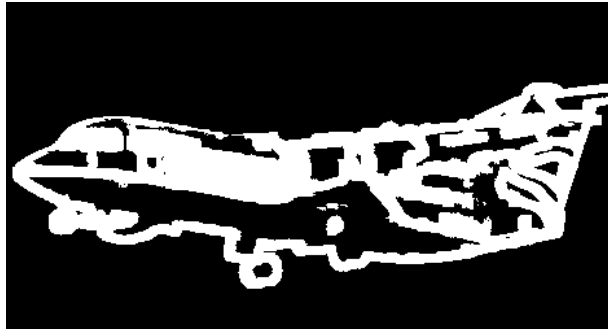
Fig. 6. Region mask created for the region-based image fusion scheme. The white areas represent “active” segments and the black areas “non-active” segments.
