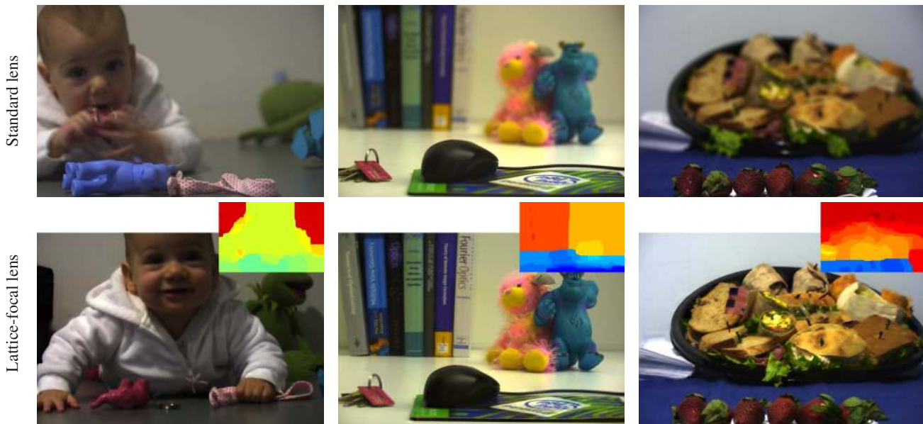
Figure 15: Partially defocused images from a standard lens, compared with an all-focused image and depth map produced by the lattice-focal lens.
