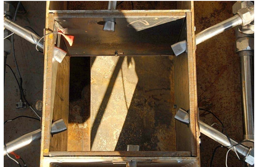
ASMAT Water Flow Testing (Below Deck Suppression Mobile Launcher Duckbill Nozzles)
