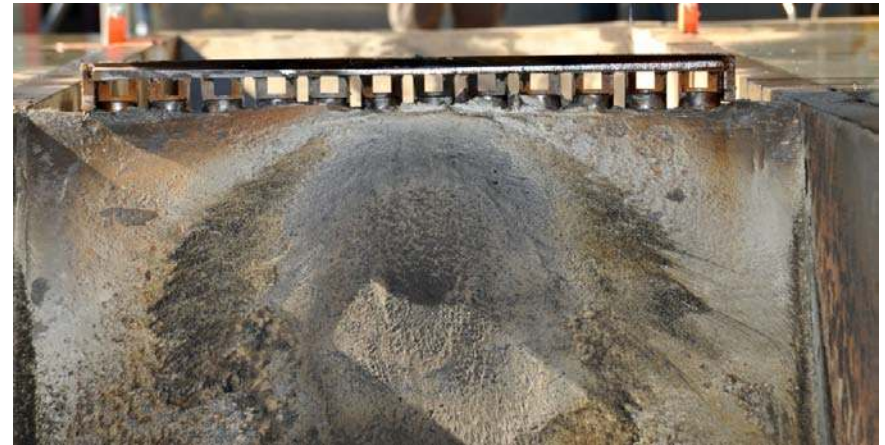
ASMAT Test IOP3 (Main Flame Deflector Crest Water Trench Suppression)
