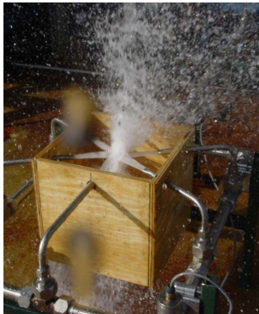
Above: Initial ASMAT water bag coverage/design
