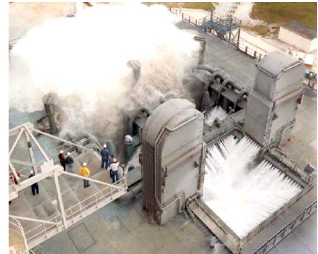
Above: KSC full-scale Shuttle MLP flow testing (2004)
