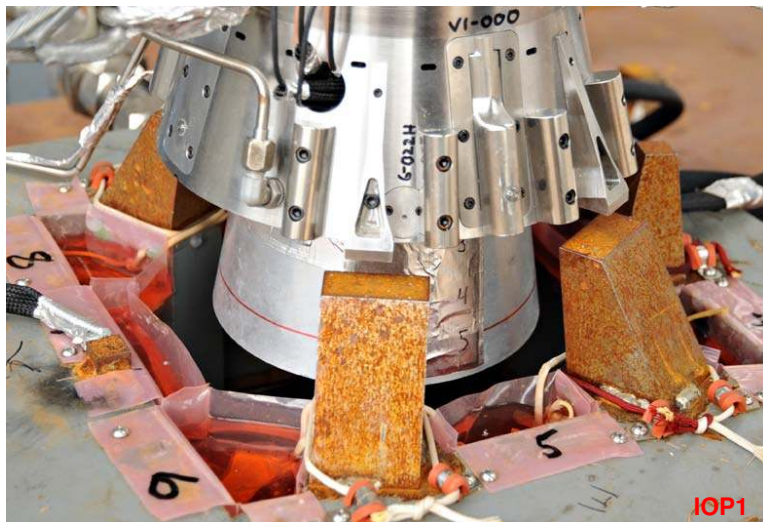
Above: Below deck IOP suppression system (ASMAT – as built) Below: Installed water bags (top view)
