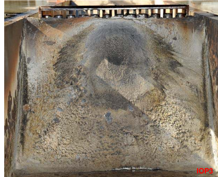
Above: Main flame deflector with crest water Below: Installed water bags and below deck IOP suppression (exhaust duct view)
