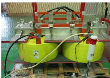
(a) MFT with alternately wound windings
