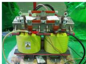
(b) MFT with normally wound windings
