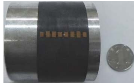
FIGURE 22: Eight-element series-fed conformal antenna array.
