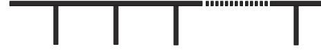
FIGURE 5: The radiating element connected with a fine line to realize the feeding.
