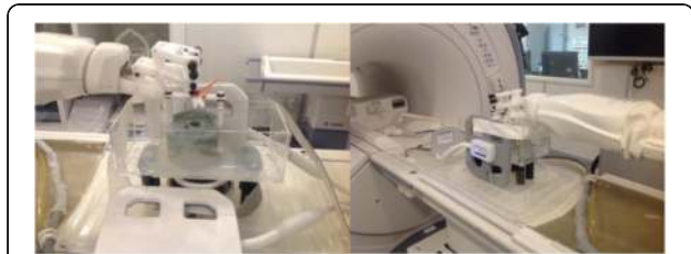
Fig. 154 (abstract A146). Experiment set up showing the phantom, phantom holder, dual flex MR coils and the INNOMOTION Robotic arm (IBSMM, Prague) to provide 1 Dimensional range of motion
