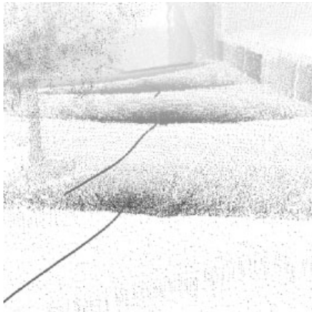
Figure 18. The trajectory after mapping shows gaps, since the robot poses are corrected at 3D scan poses.
