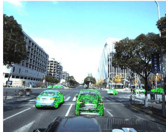
Figure 1: 6D-VNet is trained end-to-end to estimate vehicles’ six degree of freedom poses from a single monocular image. The output will precisely estimates the vehicle’s voxels in 3D occupancy.
