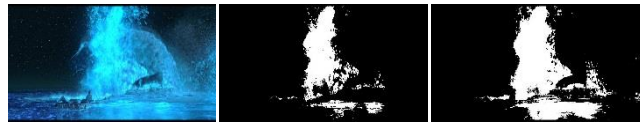
Figure 4. Clipped pixels prediction for Life of Pi: tone mapped (left), clipped pixels predicted by the PL only (middle) and predicted using both the PPL (right).
